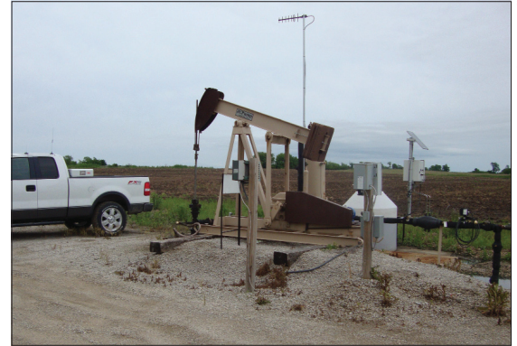
Figure 5—Coalbed methane well in Neosho County, Kansas. The electrically driven pumpjack is for drawing water from the coalbed so that adsorbed gas can be evolved from the coal. This well has a telemetered production system (note aerial) and has produced 384 million cubic feet of gas in 4 1/2 years.
