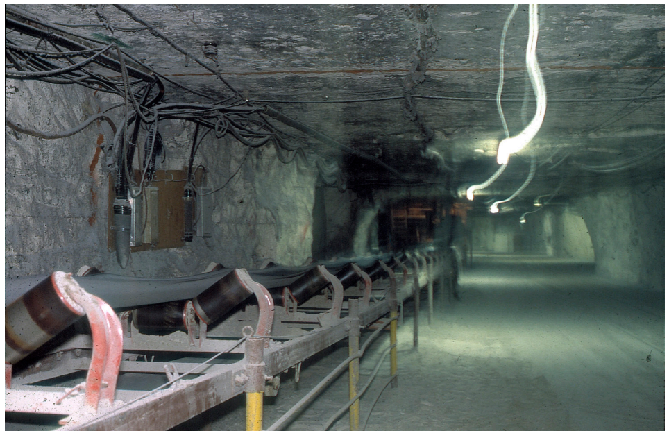
Figure 5. Underground salt mine at Hutchinson. Salt is mined in a room-and-pillar fashion and moved along a conveyor belt and eventually to the surface.
