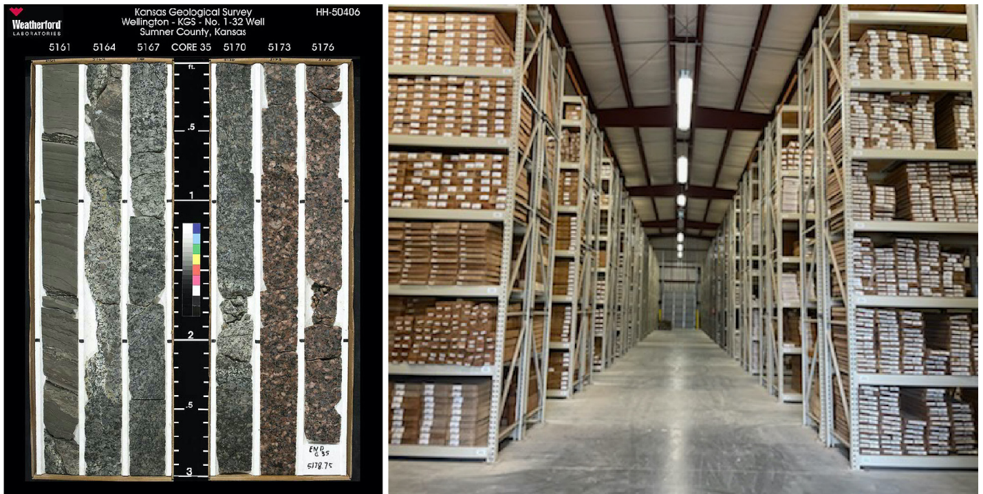
Figure 4. At left, an example of a drill core that has been cut (slabbed) and polished. At right, the KGS Drill Core Library's core storage facility.
