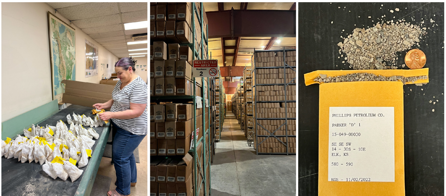
Figure 5. At left, cuttings being bagged as part of the sample curation process at the Kansas Geologic Sample Repository in Wichita. Center, one of several cuttings storage facilities in Wichita. At right, cuttings from a well in Elk County, Kansas.
